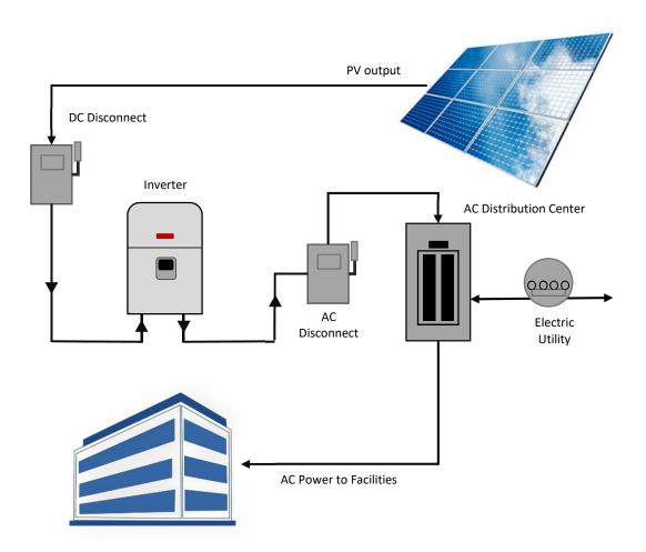
In the typical PV Grid-Tie system the PV panels generate DC power which is converted to AC power by the Inverter. Output from the Inverter is connected to your AC distribution center which feeds the rest of your Facilities.
