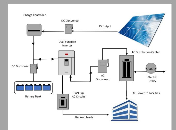
The typical Hybrid PV system incorporates a Charge controller and Dual function Inverter to create a grid tied system with a battery back-up.
